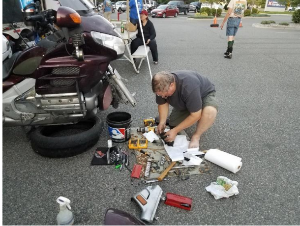
When a brake pad replacement turns into major surgery. Marc Beaulac struggling with a rounded off allen-head brake caliper pin. When all else fails, use a hammer.
