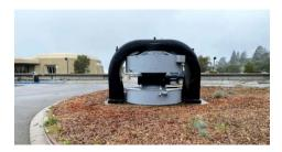
This is the electromagnet from the world's first major cyclotron. Weighing in at 85 tons, this cyclotron created the first man-made element, Technetium.
